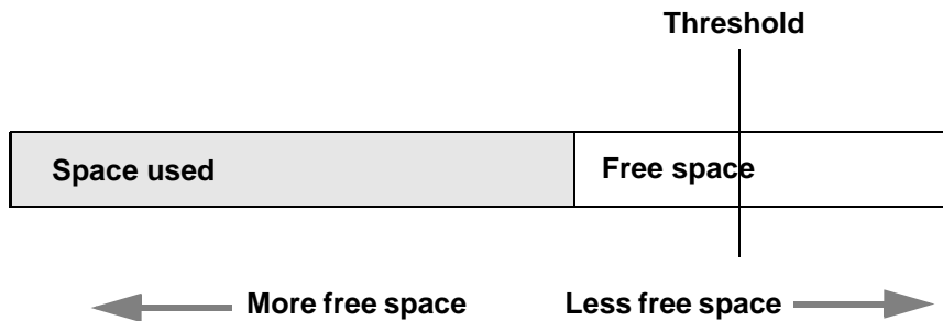
Figure 16-1: Log segment with a last-chance threshold
