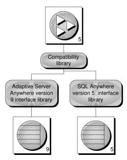
The following figure illustrates the algorithm used by the compatibility library to connect to a server:
