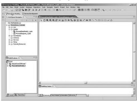
The Physical Data Model (PDM) editor displays an empty diagram and a toolbar. The **Modeling Output** view appears.
