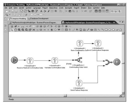
8 To change an undefined process, right-click the Receive Restock Confirmation Data process symbol and select Change to Receive from the context menu.
