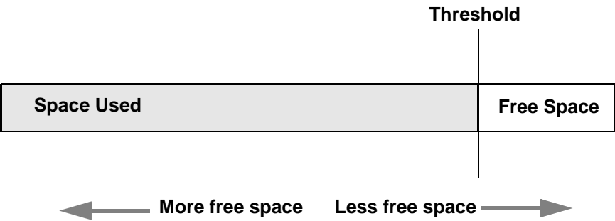
Figure 29-2: Executing sp_thresholdaction when the last-chance threshold is reached
