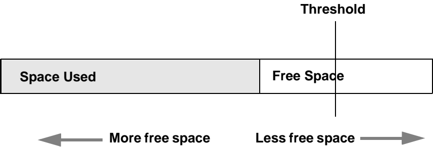
Figure 29-1: Log segment with a last-chance threshold
